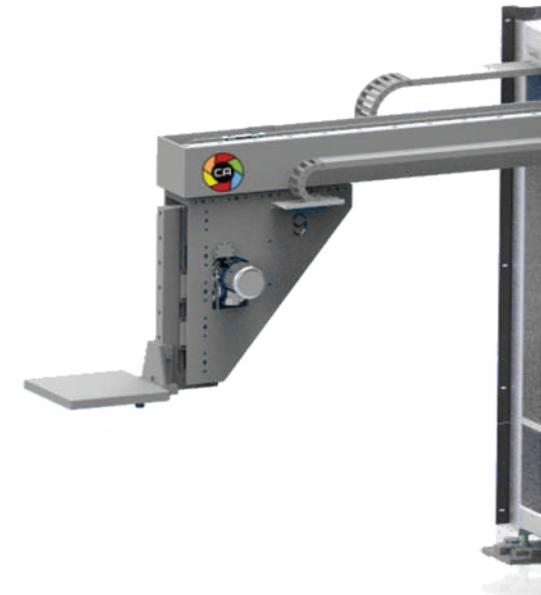
change systems with our 3, 4 and 5 axis milling machines. The main element is a structure with a non-variable volume, on which pallets of different sizes are accommodated. The quantity of the pallets that can be placed inside the "CrossArm" depends directly from the size of the pallets (CA \*\*) chosen.
